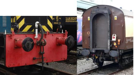
Class 04 showing screw coupling and vacuum pipe, Mark 1 coach showing buckeye coupling in the 'rest' position.
